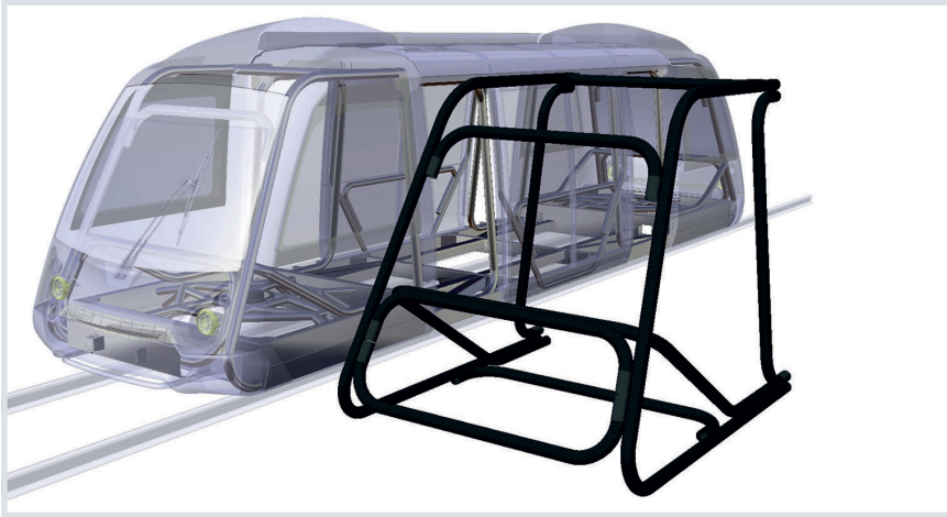
Fig. 1. Spaceframe for a metro rail vehicle front end made from braided tubes. To reduce the weight, comprehensive changes in geometry were undertaken © Far UK
